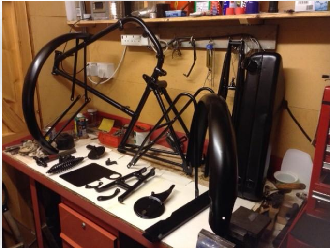
Some of the parts that have been blasted and coated.
