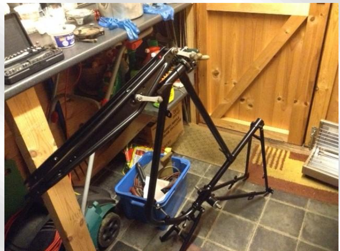
The New Hudson frame now has its stand, spindle and forks installed.
