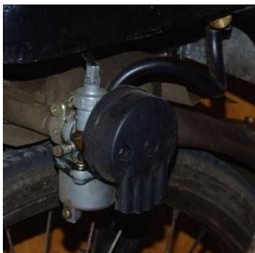
convenient were they the other way. There is a little sink in the bottom of the float chamber with a drain screw, this conveniently collects the dirt from my fuel tank. There is a spring loaded throttle stop screw.
