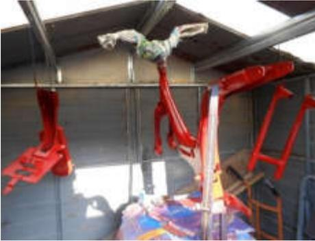
Preparation to paint also included the swing arm, rear rack plus the tops of the original shock absorbers and number plate bracket. The red chosen looked completely wrong and after just one coat I concluded the match was miles away and reordered.
