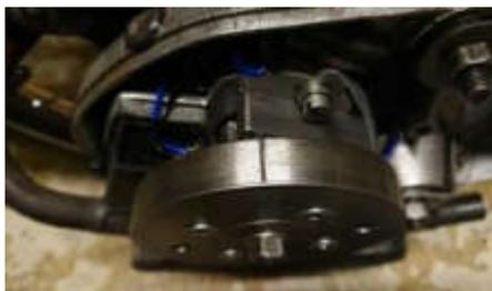
Next I put some white PVC tape on the flywheel (aligned with the TDC groove) and added timing marks in black so they would show under the strobe.
