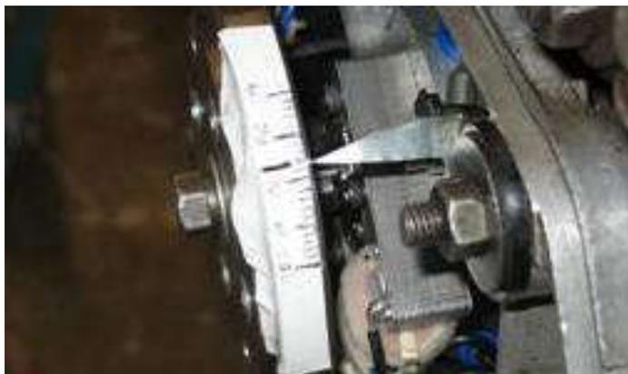
works out as 23 degrees before top dead centre (thick black line in photo above). When I used the strobe I found the CDi has a built-in automatic advance of about 6 degrees, whereas the old magneto was fixed timing.
