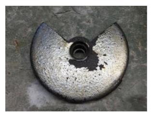
So what do you do with, picking a part entirely at random, a flywheel from a Mobylette AV76 as fitted to a cutaway display bike?
