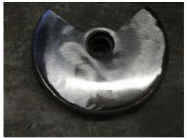
The blasting stage isn't necessary, as the first operation that starts to make a real difference is a fine grit flap disc on a 4 ½" angle grinder. Keep the flap disc moving to prevent flat spots, and keep gently sanding until all corrosion and pitting has been removed. Now for the magic to start.....
