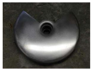
Staying with the orbital sander a 320 grit paper is used to further refine the surface, and remove any remaining scratches from the flap disc stage.
